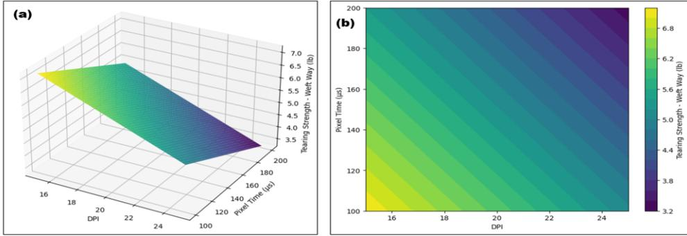
**Figure 3.** (a) 3D surface and (b) contour plots for tearing strength in the weft direction
