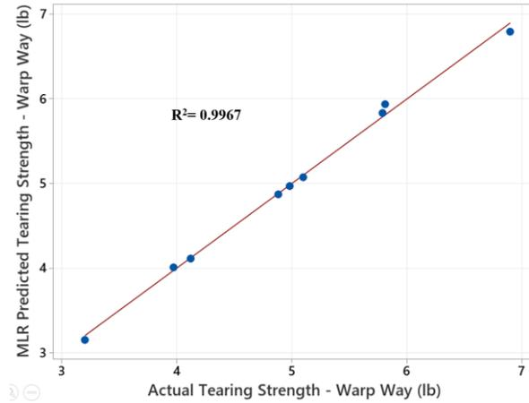
**Figure 5.** Correlation between actual and predicted values of Tearing Strength (warp way)
