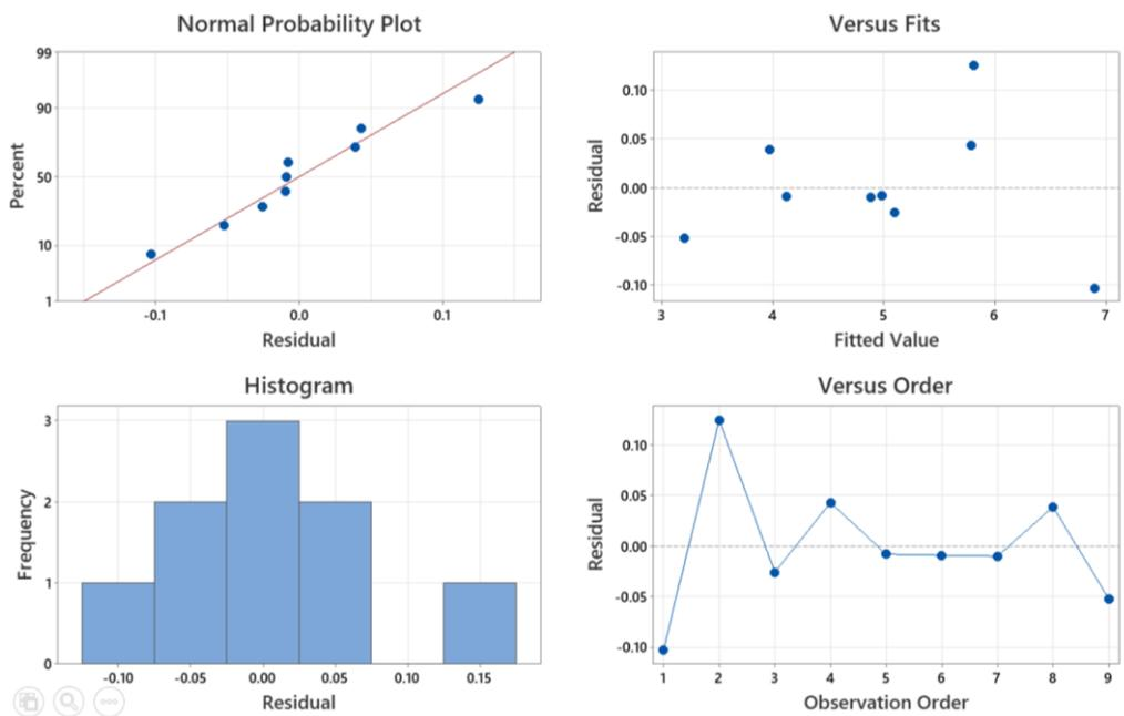
**Figure 9.** Residual plots for the MLR model (warp way)
