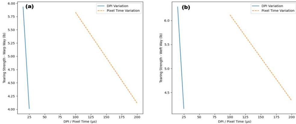
**Figure 1.** Sensitivity of tearing strength to variations in the input parameters, Dot Per Inch (DPI) and Pixel Time, ( a) warp way (b) weft way
