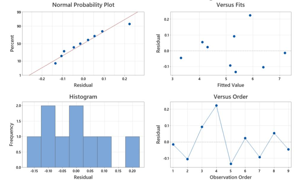
**Figure 10.** Residual plots for the MLR model (weft way)
