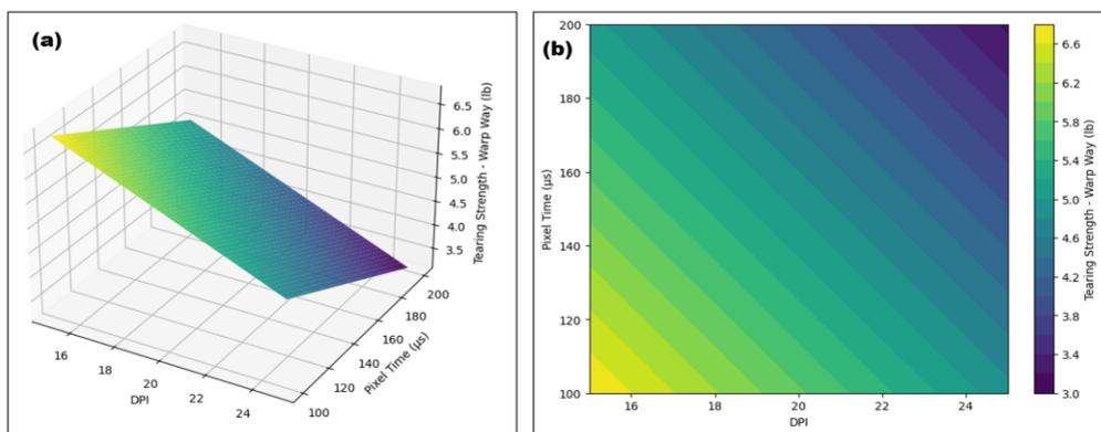
**Figure 2.** (a) 3D surface and (b) contour plots for tearing strength in the warp direction
