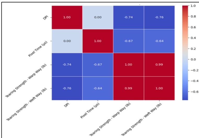
**Figure 4.** The correlation matrix heatmap, which shows the relationships between Dot Per Inch (DPI), pixel time, and the tearing strength
