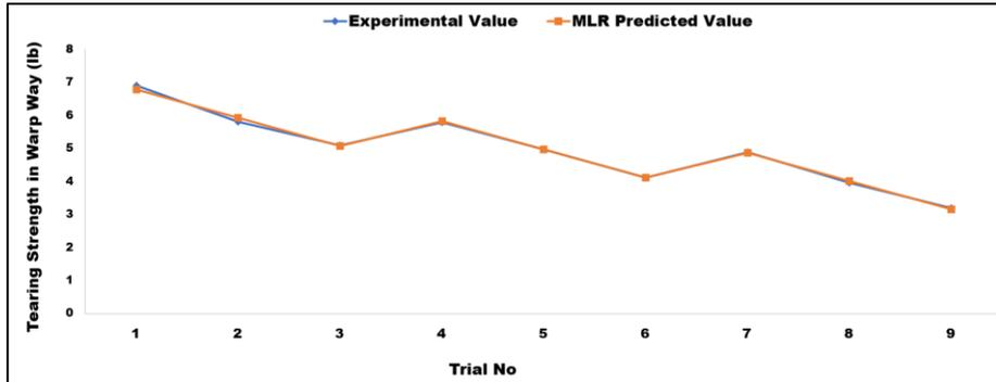
Figure 7. Comparison between the experimental values and MLR predicted values with line diagram for tearing strength in the warp directions
