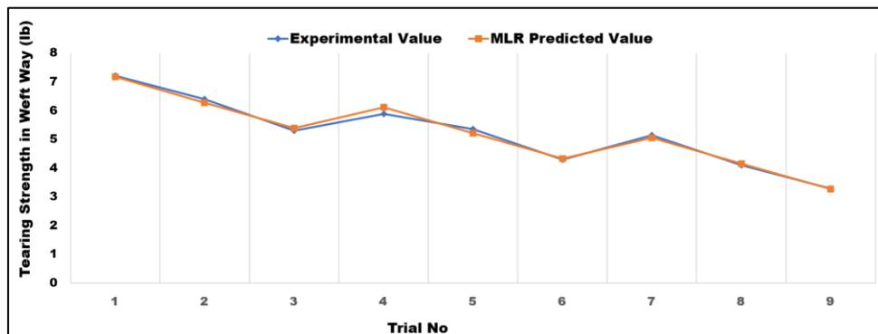
**Figure 8.** Comparison between the experimental values and MLR predicted values with line diagram for tearing strength in the weft directions
